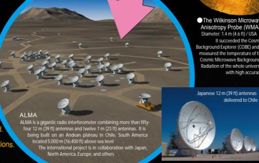
ALMA is a gigantic radio interferometer combining more than fifty-four 12 m (39 ft) antennas and twelve 7 m (23 ft) antennas. It is being built on an Andean plateau in Chile, South America located 5,000 m (16,400 ft) above sea level. The international project is in collaboration with Japan, North America, Europe, and others.
