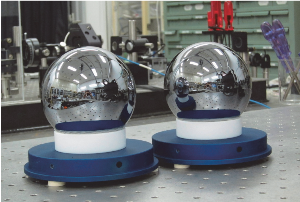
Enriched silicon sphere used for determination of Planck Constant
