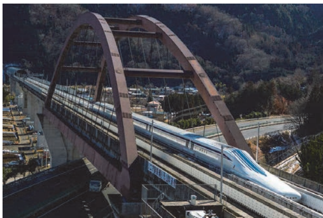
Superconducting maglev train running on the Yamanashi test line
