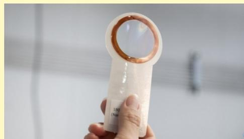
CO<sub>2</sub> permeable membrane of 34 nanometer
