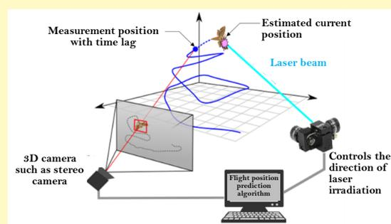
Schematic diagram of pest control system by laser sniping
