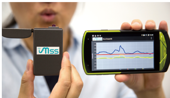
Breath measurement using an olfactory sensor (source: National Institute for Materials Science)
