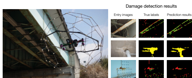
Autonomous drone and technology to automatically detect damage in structures based on deep learning under development (source: RIKEN and Tohoku University)
