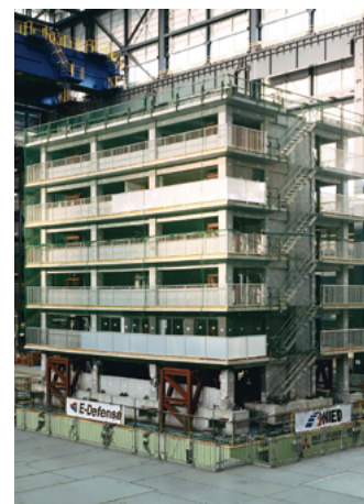
3D Full-scale Earthquake Testing Facility (E-Defense) (source: National Research Institute for Earth Science and Disaster Prevention)
