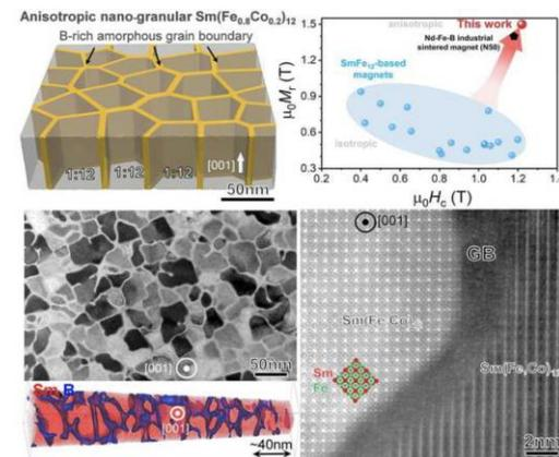
Sm(Fe<sub>0.8</sub>Co<sub>0.2</sub>)<sub>12</sub>-B film with  $\mu_0 H_{cJ} = 1.2\text{T}$
