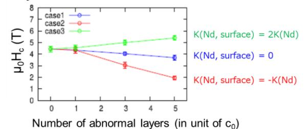
Dependence of coercivity on numbers of atomic layers from surface of  $\text{Nd}_2\text{Fe}_{14}\text{B}$  in which magnetic anisotropy of rare earth ions are manipulated.
