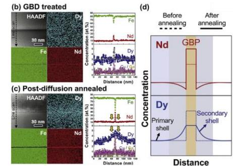
Microstructure and distribution of Dy in the outermost skin of main phase grains in Dy-GBD treated Nd-Fe-B sintered magnet of  $\mu_0 H_{cJ} = 3 \text{ T}^{-1}$
