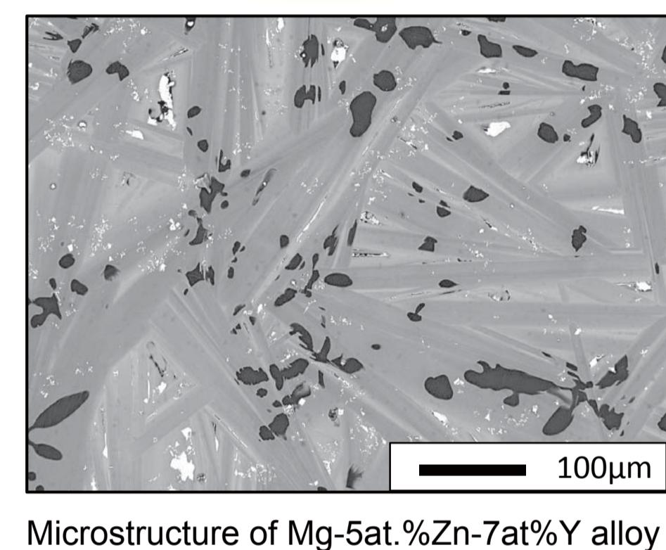
Microstructure of Mg-5at.%Zn-7at%Y alloy
