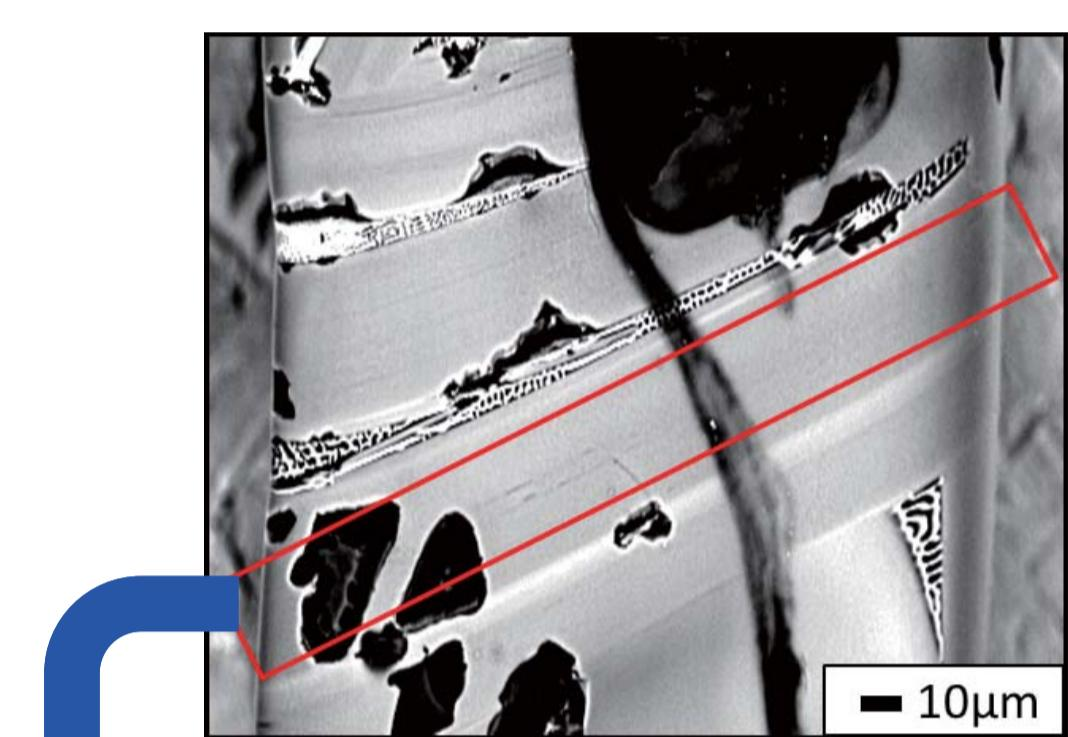
A small single crystal was cut out (20 X 30 X 100  $\mu\text{m}^3$ )
