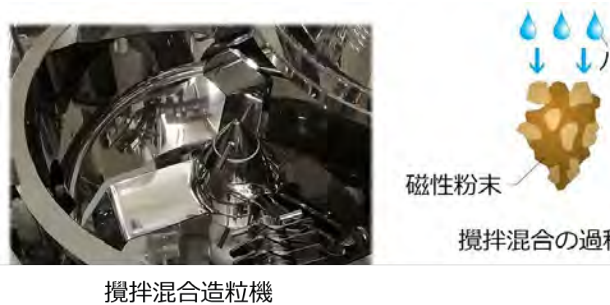
Figure 2.1.3.5 Binder granulation process
