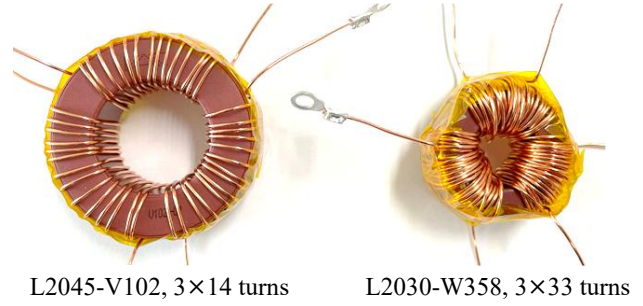
Figure 1.3.2.12. Appearance of the fabricated CMI (Left: with high permeability core, Right: with low permeability core)
