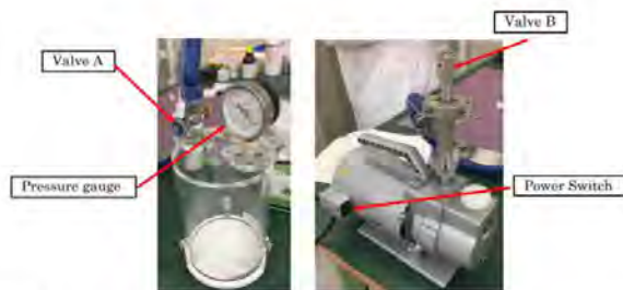
図2-2 九工大の真空引き装置(引用:Solar Cells Attachment Procedure and its verification method)
