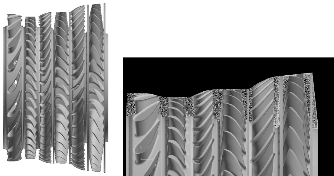
Fig. 2.2.4-9 Geometry and mesh of turbine.
