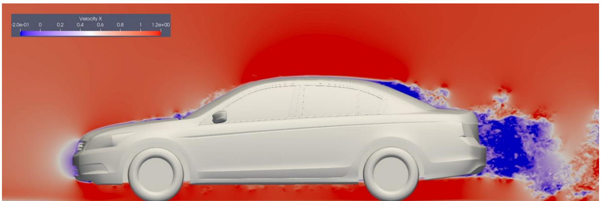
Fig. 2.2.5-20 Flow field around an automobile simulated by FFX, Re=Re_0/40 .
