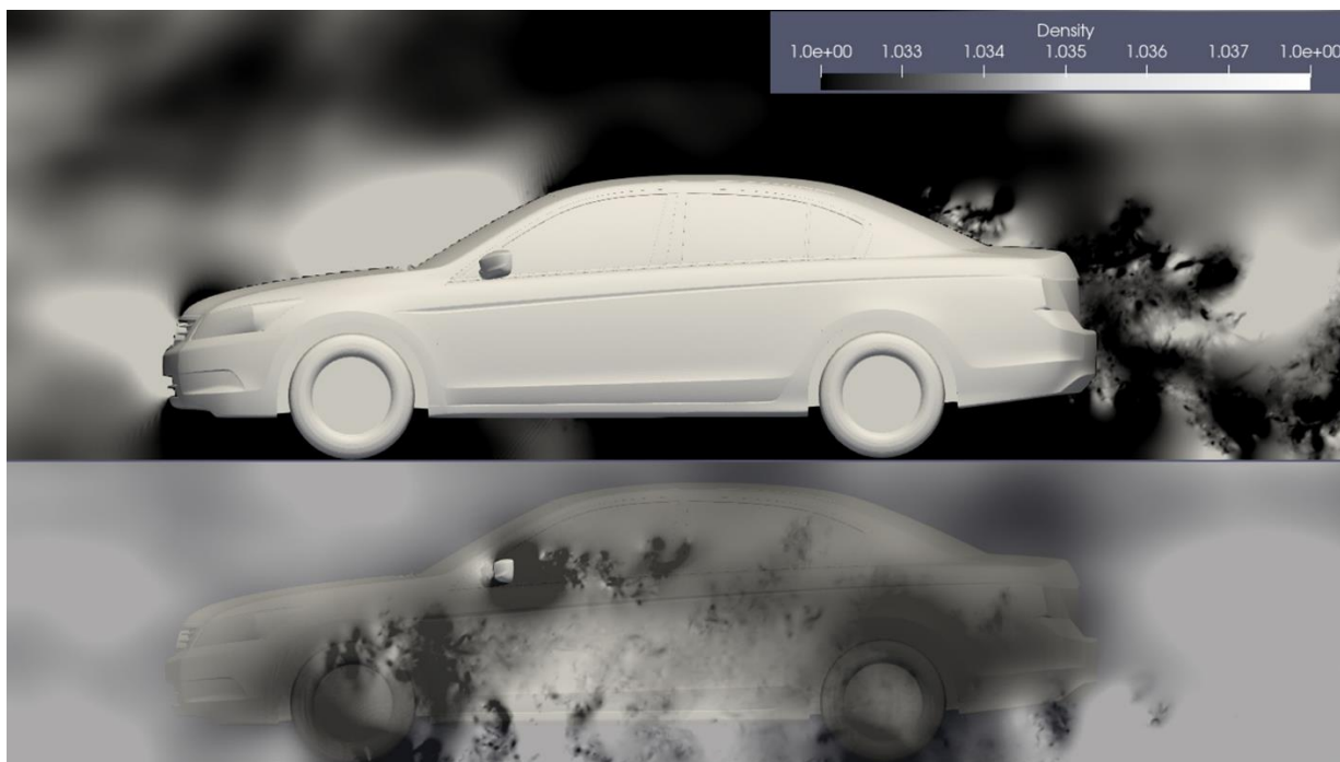
Fig. 2.2.5-24 Sound fields around an automobile simulated by FFX, Re=Re_0/40 .
