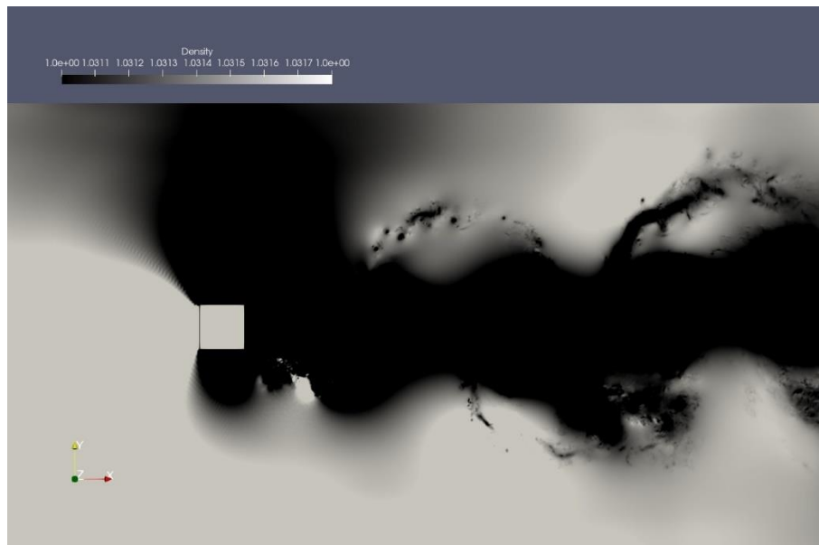
Fig. 2.2.5-12 Density field around a square cylinder.
