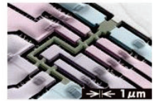
Figure 3. Single-crystalline sample micro-fabricated by FIB to measure transport properties.
