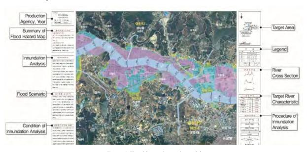
Figure 9 Flood hazard map (sample)
