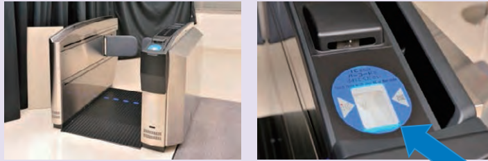
Figure 1 / Boarding Gate with a Built-in Explosives-Detection Apparatus
