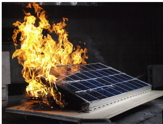
Fire exposure experiment of a solar cell module
