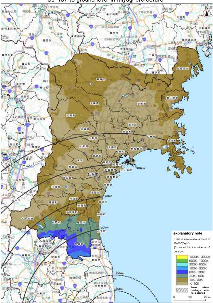
Results of aircraft monitoring by MEXT and Miyagi Prefecture (Total surface deposition of Cs-134 and Cs-137 inside 100 and 120 km zone of TEPCO Fukushima Dai-ichi NPP and in northern
