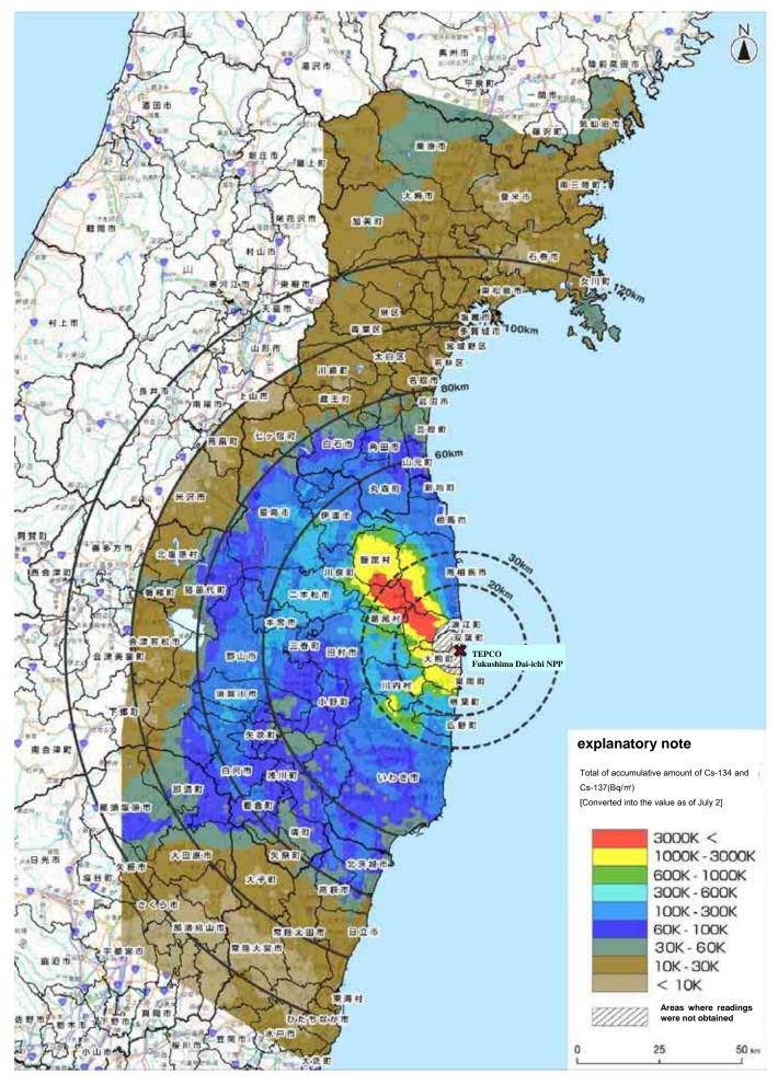
Results of aircraft monitoring by MEXT and Miyagi Prefecture (Total surface deposition of Cs-134 inside 100 and 120 km zone of TEPCO Fukushima Dai-ichi NPP and in northern
