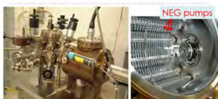
Our "Load-locked" GaAs photogun: • Gun Vacuum ~ mid to low 10^{-12} Torr • Large Grain Niobium Electrode
