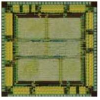
A system LSI chip contains processors, memories, communication interface circuits, and analog circuits, which are integrated on a small silicon chip. It is used in various electronic devices.
