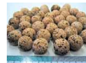
Filtering materials made from Akita cedar charcoal and zeolite
