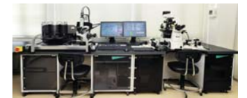
The system to collect and analyze nucleated red cells in the blood
