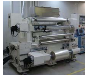
Roll-to-roll typed system for DLC films by high-speed atmospheric pressure plasma CVD technique
