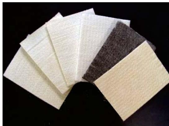
Photocatalytic mats with various characteristics
