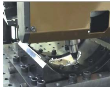
Fig. ③/Operation of FSW on three-dimensionally curved surfaces
