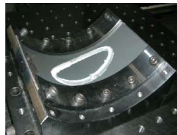
Fig. ④/Example of a tilted elliptic path followed by FSW inside a quarter-cylindrical plate
