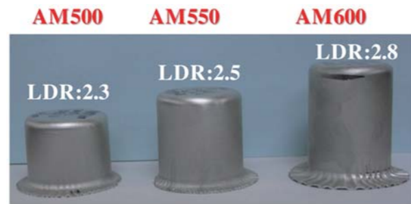
Press-forming Parts Using the Developed Material
