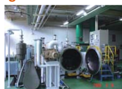
Figure 1 (a) Vacuum melting furnace in the Kamaishi Area
