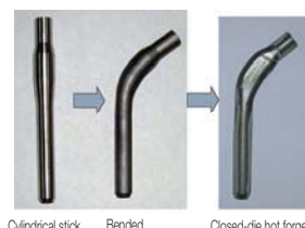
Figure 3 Artificial hip joint made of Ni-free Co-Cr-Mo alloys following the net-shaped closed-die forming technique
