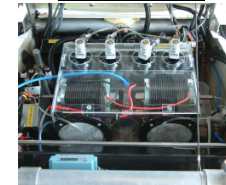
150W Fuel Cell and Hydrogen Absorption Alloy Cylinders
