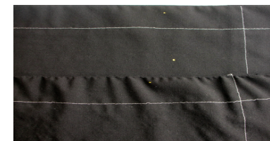
Upper slide: material processed with slide ring technique, washed 20 times. Lower slide: Untreated material, washed 20 times.
