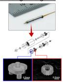
World's smallest & high sensitivity pressure sensor for automobiles using BMG
