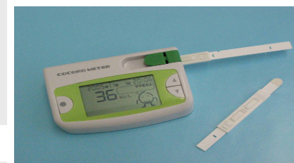
(b) The marketed stress measure (Nipro Corp., COCORO METER, 130 × 87 × 40 mm 3 )
