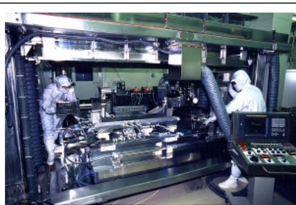
数値制御EEM(Elastic Emission Machining)装置
