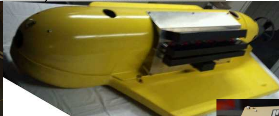
Hydrophone array : 80cm long, 48ch, 4 rows × 12 elements
