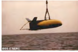
The deep tow boomer was developed by BGS to further enhance their seismic suite of tools to gain high-resolution images from deeper targets. The tool can operate in water depths of down to 2000 m and as shallow as 100 m. The boomer has a penetration of up to 150 m sec with a resolution of 1 ms or less. The idea is based on towing both source and streamer closer to the sea bed, (higher along track resolution) and in an acoustically quiet environment found at depth.
