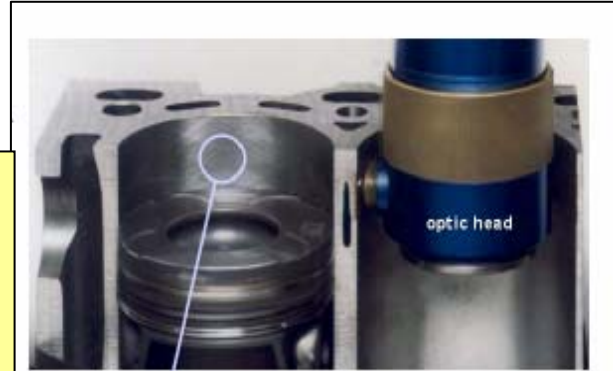
Fig. 16: Microstructuring of engine cylinder walls (by courtesy of FGSW (Fa. Gehring GmbH resp.))
