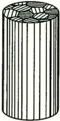
Schematic illustration of DS TiAl (M. Yamaguchi)
