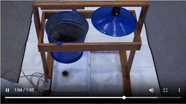
The video displays a Tullgren apparatus, a common tool for soil animal extraction. It consists of a wooden frame with two blue buckets on top. A clear container is placed below the buckets to catch any animals that fall through. The video shows the apparatus in use, with a small amount of soil visible in the clear container. The video player interface shows a progress bar at 1:04 / 1:35.
