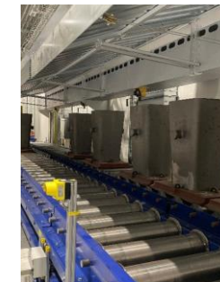
Mould handling line
