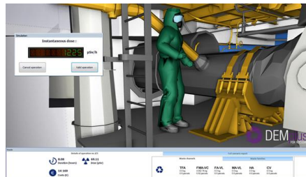
DEMplus® simulation of different scenarios for large components treatment (pressurizers), in-situ cutting/conditioning or off site treatment → comparison in terms of dosimetry, waste volumes, schedule, costs...
