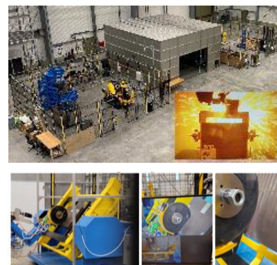
Tests on several teleoperated cutting techniques
