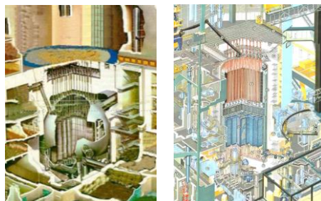
The complex design of French UNGG (Chinon A2 and Saint Laurent reactors)
