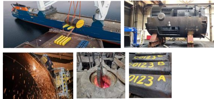
Feasibility demonstration of Fessenheim's used SGs upper parts treatment and recycling
