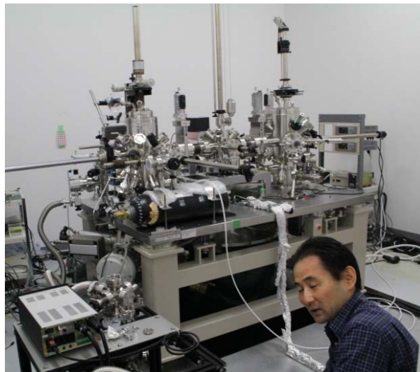
Figure 1: Dr. Hitosugi, AIMR, and his special STM, the optical axis of which was seriously damaged by the earthquake.
