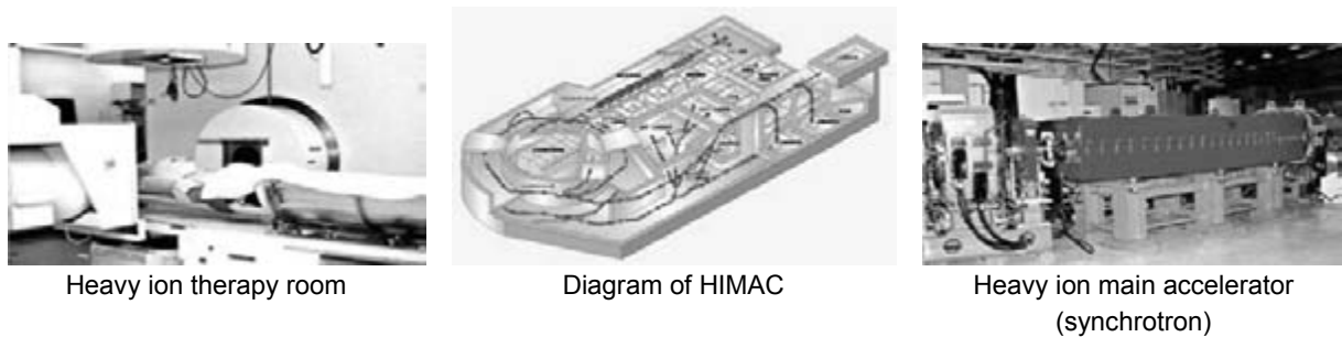
Figure 1-1-17 Heavy ion cancer therapy system (HIMAC)
