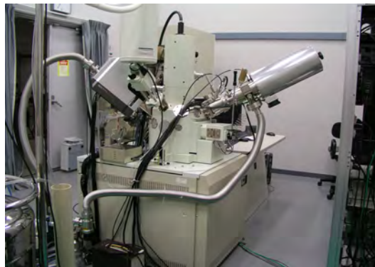
Advanced measurement/analysis instrument (X-ray analysis system for light elements of materials by low-energy ion irradiation)
