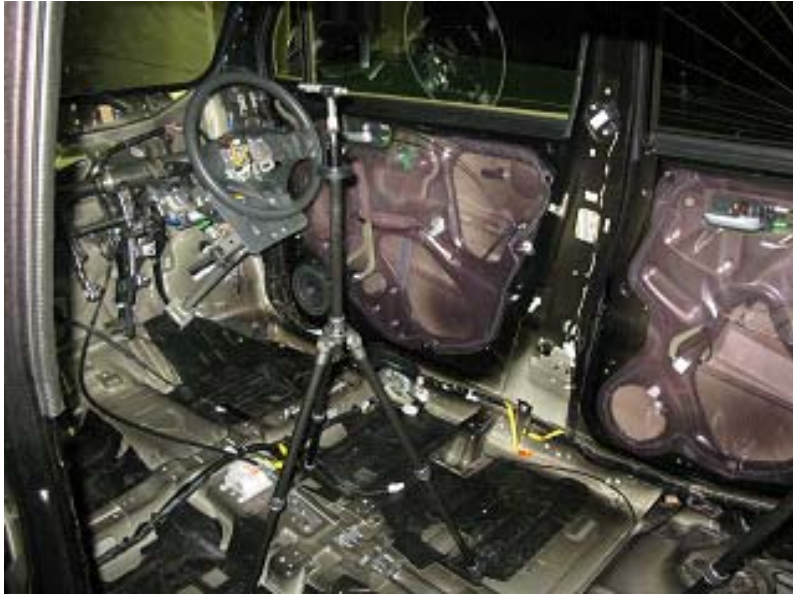
Fig.3-35 Picture of the interior of automobile for wind tunnel experiments. Interior panels and the seats were removed to eliminate the sound absorbing effect in experiments.
