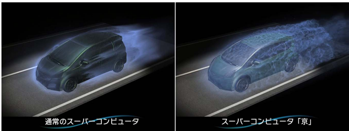
Fig. 3-17 Wind Tunnel full vehicle aerodynamics LES simulation using unstructured 4.8 billion elements. Top, vehicle geometry and suspension-tire configuration: middle, empty wind-tunnel pressure gradient(left) and a result example of velocity field(right) ; bottom, comparison of the conventional simulation using RANS model with 55 million elements (left) and the high-resolution simulation using LES with 3.5 billion elements on the K-computer(right).
