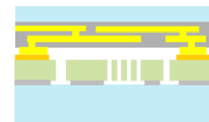
(e) VHF released and hermetic wafer bonding
