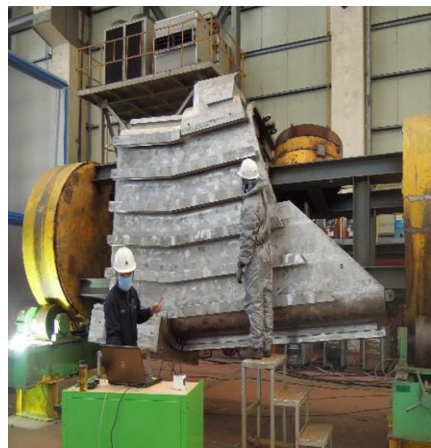
T-rib to Inner Shell ass'y of LPSE
