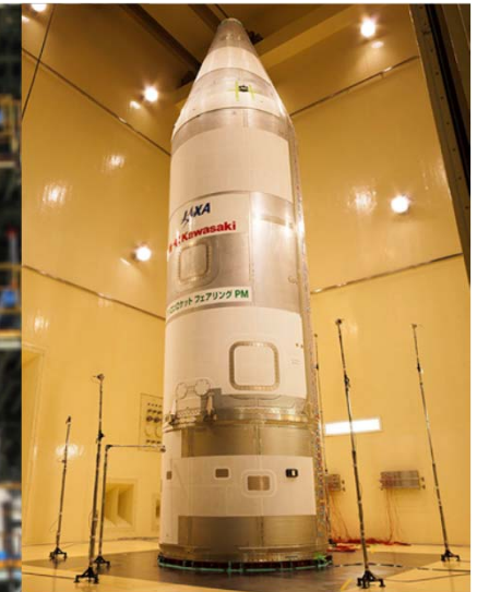
PM音響試験@JAXA TKSC
