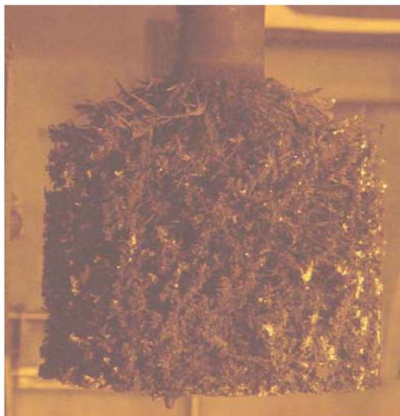
Figure 3. A cathode removed from Mk-IV ER, 10.1 kg
