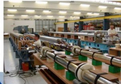
Assembly of 15 m long coils in industry, 2003
