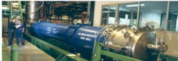
First LHC dipole prototype on the test bench (June 1994)
