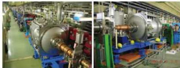
Fig. 5-3-1-9 KEKB superconducting crab cavities. (left) Crab cavity for HER and (right) crab cavity for LER.
